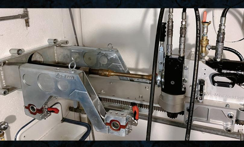
The MiniRockDrill can be easily and quickly placed in the house/cellar/garage to the P2O wall bracket or to a core hole wall bracket. As the unit consists of two main parts, a simple and quick installation is guaranteed, even in confined spaces and with minimum component weights. With our optional DN2OO corehole wall bracket, the installation is even faster directly in the core hole.
