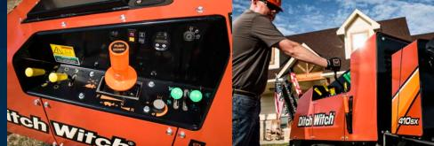
The Ditch Witch® 410SX is the most outstanding articulated-steer vibratory drop plow in its horsepower class. With dozens of innovative features, including an oscillating rear axle that keeps the machine's fourwheel drive engaged, the 410SX quickly and efficiently installs communication lines, natural gas and water services, or a complete underground sprinkler system without digging a trench. Need a trench? The 410SX can do that, too.
