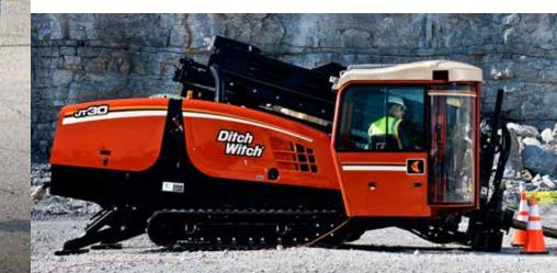
Heavy-duty stakedown system allows you to push or pull with full machine thrust and remain secure in virtually any drilling condition.
