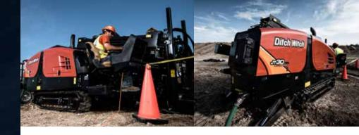
Open-top vise wrenches are angled toward the operator for an excellent view of the tool joint when making up and breaking out pipe.
